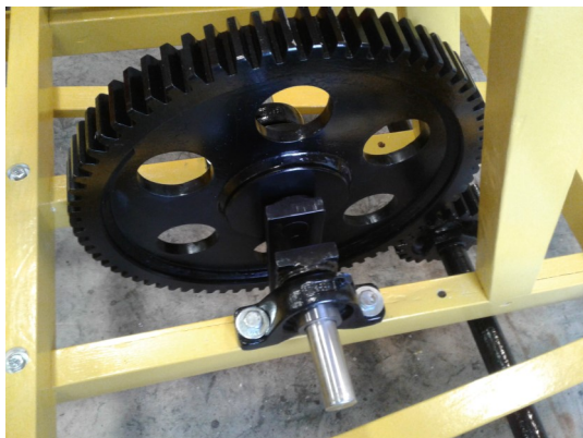
Photo (Left): One of the main components that we had to out-source was the main 72 teeth drive gear weighing in at 86lbs. This is the S472 Martin Gear from original pump cars based on the plans we have. The gear was ordered from Martin Gear in Canada but came from a plant in Texas.
